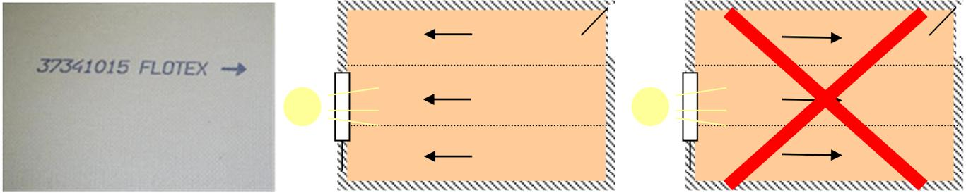
Measure the area to be installed and determine the direction in which the material will be installed and seam placement. Seams must be a minimum of 15 cm away from any subfloor joints such as day joints, saw cuts, etc.
