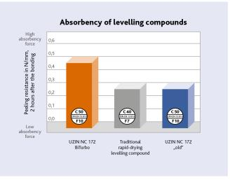
The absorption capacity of UZIN NC 172 BiTurbo is approx. twice as high as usual rapid-drying levelling compounds. The open time of the adhesive during the laying is considerably reduced in comparison with usual compounds. The overall appearance of the finished floor covering surface is very smooth and flat.
